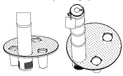
c. Drop the brine grid with brine well inside the brine tank such that the nut fitting faces the hole on the brine tank. Then press the grid evenly inside the brine tank until the brine grid legs touches the bottom of the brine tank.
