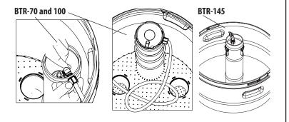
**f.** For installation of brine tank at the installation site, pull the other end of the brine tube from the hole on the brine tank. The completed assembly is shown below:
